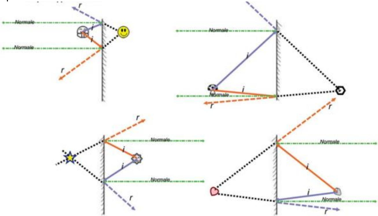
For a bigger more complicated object use the « trick with the normal » to find the image of several points on the object, and then draw the rest of the image
