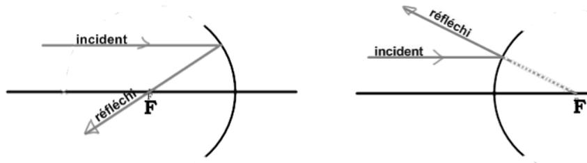
Incident rays through the focal point -----> Reflect parallel
